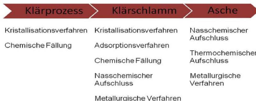
Figure B: General overview of options for phosphorus recovery
